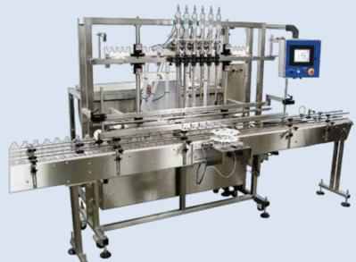
Linear Servo Pump based Filling Machine
